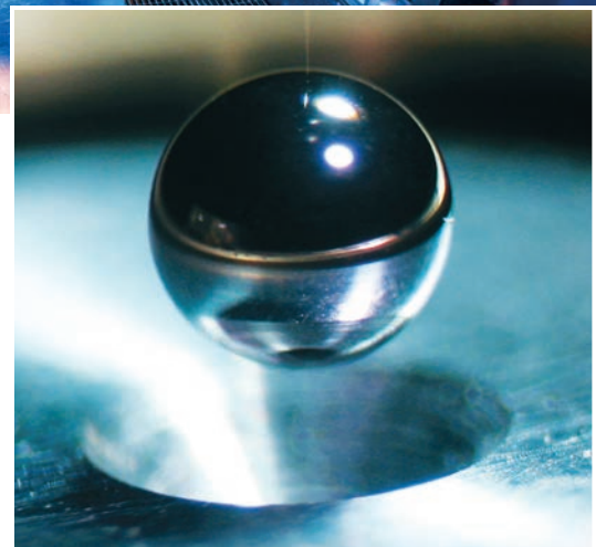
A two-millimeter-diameter capsule filled with a deuterium-tritium (DT) gas, surrounded by a few-nanometer-thick layer of DT ice, which is the target for the lasers of the National Ignition Facility.
