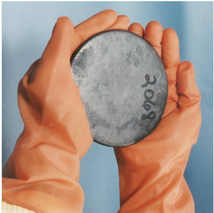
The Y-12 Plant in Oak Ridge, Tennessee, converts uranium-235 powder to metal discs or “buttons,” which are then manufactured into weapons components.
