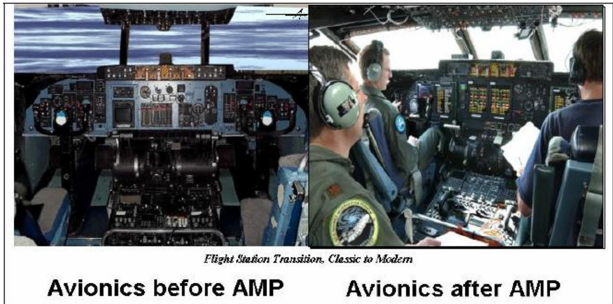
Figure 3. Cockpit from the original program compared to AMP (Griffin, J).
