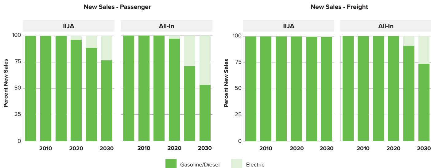
FIGURE 3 | New passenger EV sales reach 23% and 47% under IIJA and All-In scenarios, respectively. New freight EV sales are less than 1% and 26% under IIJA and All-In scenarios, respectively.
